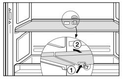
Press down on the hook ① underneath the rear of the separator shelf and pull the shelf forwards and out ②.
